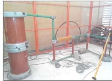
Fig.4. Dielectric strength test equipment
